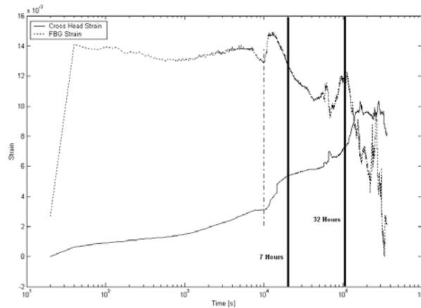
Figure 1: Strain vs. Log(Time) curve obtained under 20 N constant load for 100 hours
