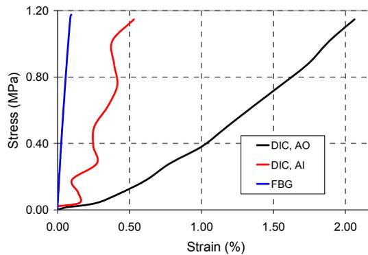
Figure 6 Stress-strain behaviour of specimen with FBG attached with Araldite 2015 adhesive
