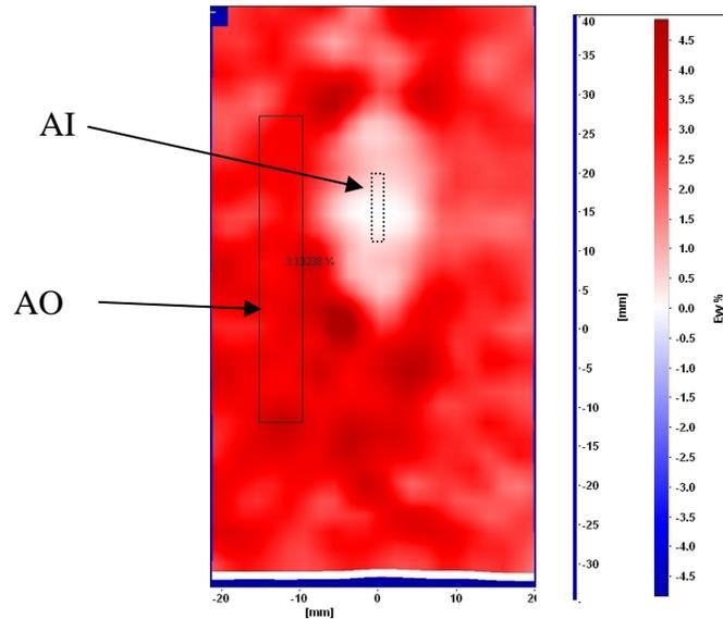
Figure 4 Longitudinal strain for specimen with FBG bonded with DMC2
