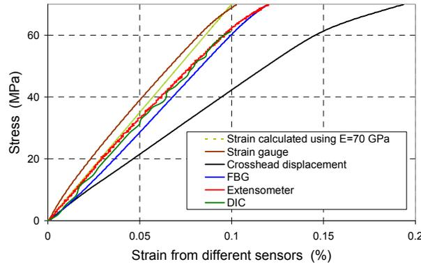
Figure 2 Stress-strain behaviour as recorded by the different sensors
