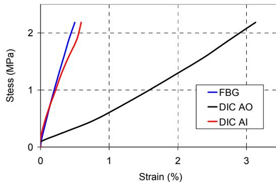
Figure 5 Stress-strain behaviour of specimen with FBG attached with DMC2 adhesive
