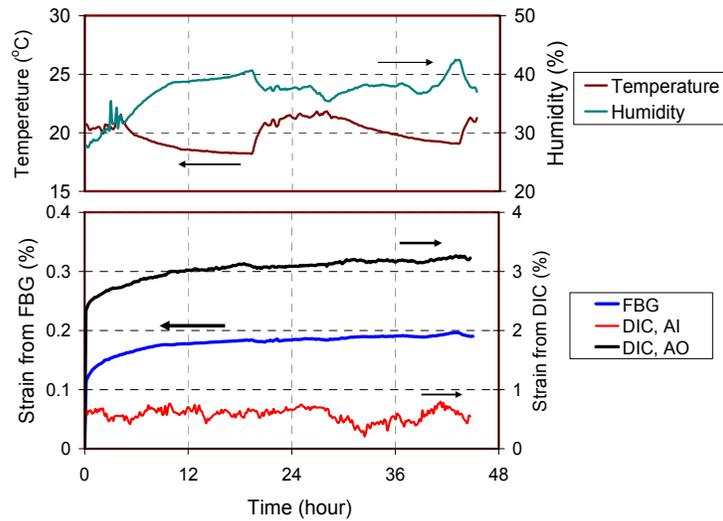
Figure 8 Results from long term test on textile specimen with FBG bonded with Araldite
