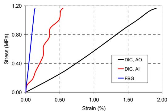
Figure 7 Stress-strain behaviour of specimen with FBG attached with Vinamul adhesive
