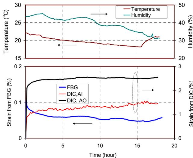
Figure 9 Results from long term test on textile specimen with FBG bonded with Vinamul
