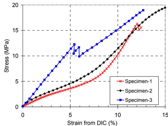
Figure 3 Stress-strain behaviour of textile with and without optical fibre
